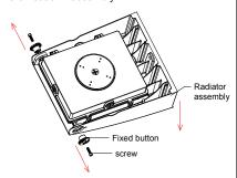
2. Use a screwdriver to remove the screw and remove the outer casing.
