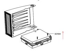
3. Unscrew the cover of the entry hole on the lamp base and remove the cover.
