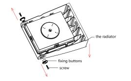
2. Unscrew to remove the fixture shell. screw
