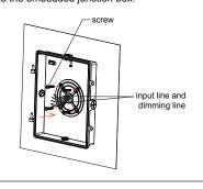
7. Install the upper half of the fixture on the lamp base, then use the threaded terminal to connect L/N/ ground wire, dim+/dim-(if not, please ignore) separately,and then plug the threaded terminals into the embedded junction box, adjust the switch to the color temperature and wattage needed.
