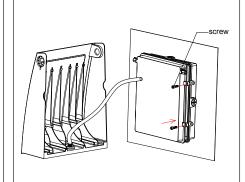
9. Install the heat sink assembly and tighten the screws and fixing knob with a screwdriver to complete the installation.
