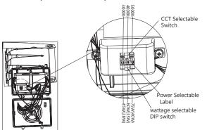
3.2.After the wiring completed, set the CCT and power value through the internal DIP switch. According to the label.
