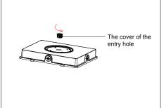
4. According to the embedded terminal box, punch the correspongding mounting hole on the light's mount.
